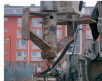
Water and binder are fed through separate nozzles on the tool.
